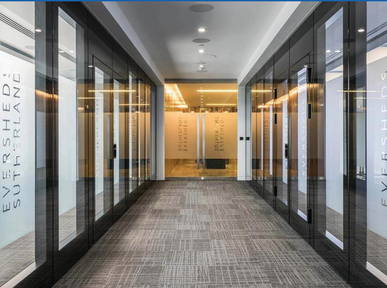
The Type RG Plus movable wall system is top-hung with double glazed frame panels, available with manual or semi-electric operation and is an ideal flexible space solution where transfer of light and optimum acoustic performance is important.
